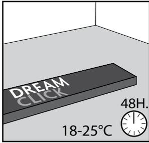
Keep the panels in the unopened package at room temperature for at least 48 hours before you start the installation. Stack horizontally in the fitting location, decorative side up. The ideal indoor climatic conditions are 18-25°C. Maintain this temperature during installation as well.
